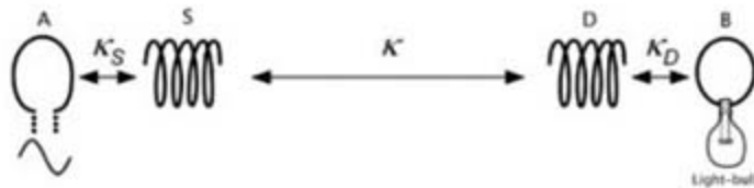
Fig. 1. Schematic of the experimental setup. A is a single copper loop of radius 25 cm that is part of the driving circuit, which outputs a sine wave with frequency 9.9 MHz. S and D are respectively the source and device coils referred to in the text. B is a loop of wire attached to the load (light bulb). The various \kappa s represent direct couplings between the objects indicated by the arrows. The angle between coil D and the loop A is adjusted to ensure that their direct coupling is zero. Coils S and D are aligned coaxially. The direct couplings between B and A and between B and S are negligible.
